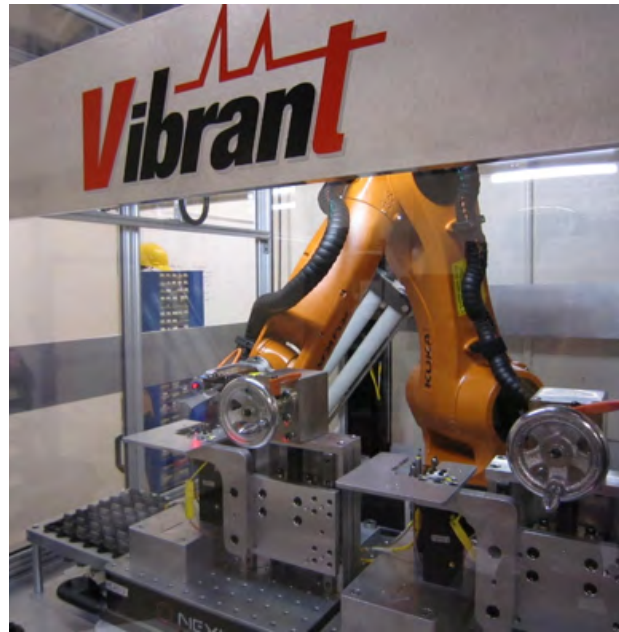
Figure 2 —Fully-Automated PCRT system. Handles higher volumes with less labor. Reduces risk of human factor inspection errors.
