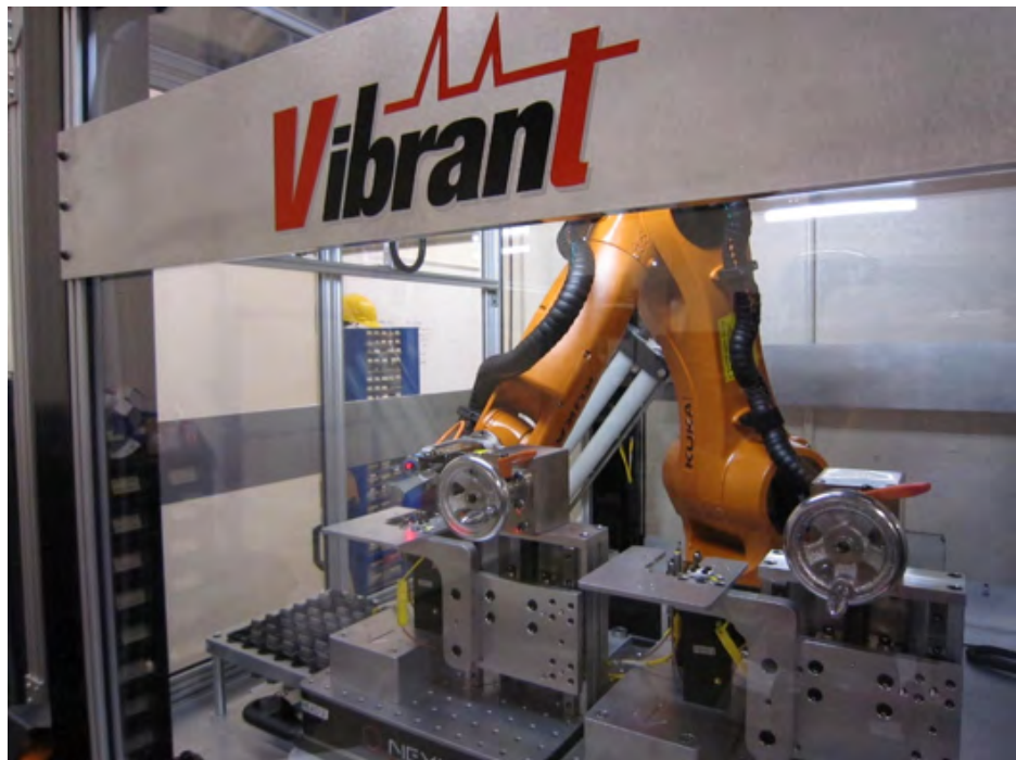
Above —Fully-Automated PCRT system. Handles higher volumes with less labor. Reduces risk of human factor inspection errors.
